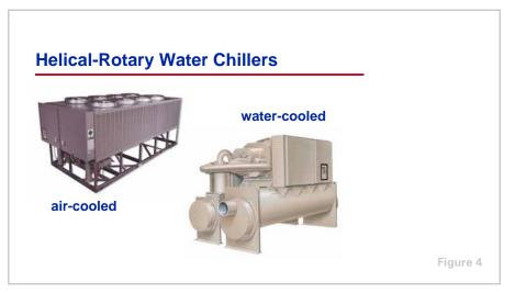
Helical-rotary water chillers can be either air-cooled or water-cooled, referring to the method of rejecting heat to the atmosphere. Both air-cooled and water-cooled helical-rotary chillers are generally available from 70 to 450 tons [200 to 1500 kW].
